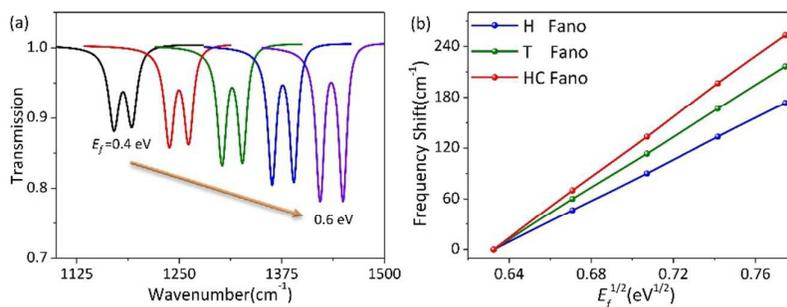
**Fig. 4** (a) Simulated transmission spectra of the HC Fano resonance structure with  $E_f$  varied from 0.4 eV to 0.6 eV. (b) The peak frequency in transparency window of H, T, and HC Fano resonance modes in the transmission spectra as a function of  $E_f^{1/2}$
