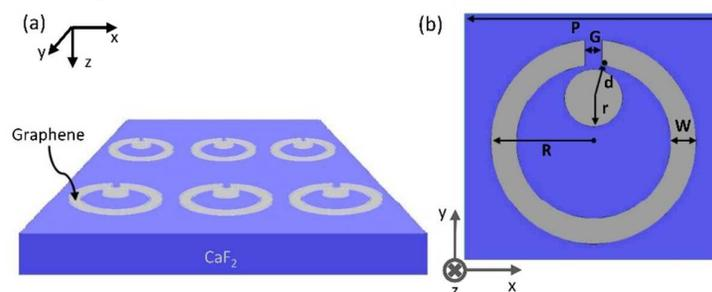
**Fig. 1** (a) Schematic of the graphene metamaterial comprised of a disk and a SRR in a unit cell. (b) Top view of a unit cell: fixed periodicity  $P = 300 \text{ nm}$ , outer radius  $R = 120 \text{ nm}$ , width  $W = 30 \text{ nm}$ , and gap  $G = 20 \text{ nm}$  of the graphene SRR, and the closest separation distance  $g = d - r$  of graphene disk and SRR.
