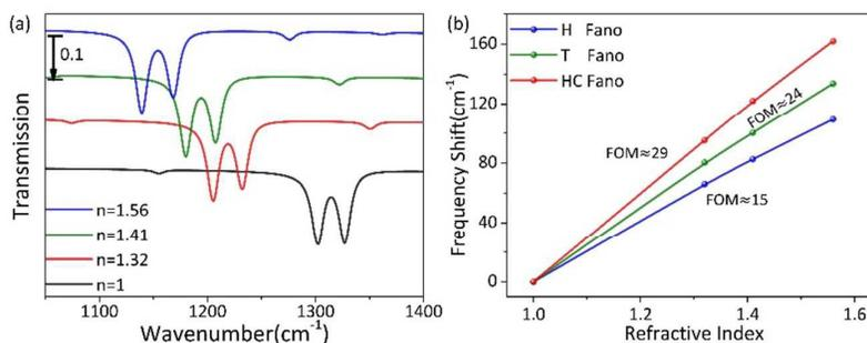
**Fig. 3** (a) Simulated transmission spectra of the HC Fano resonance mode with different analytes (marked by refractive indices). (b) Frequency shift of H, T, and HC Fano resonance modes versus the refractive index of the analyte. The corresponding FOM values are also shown.
