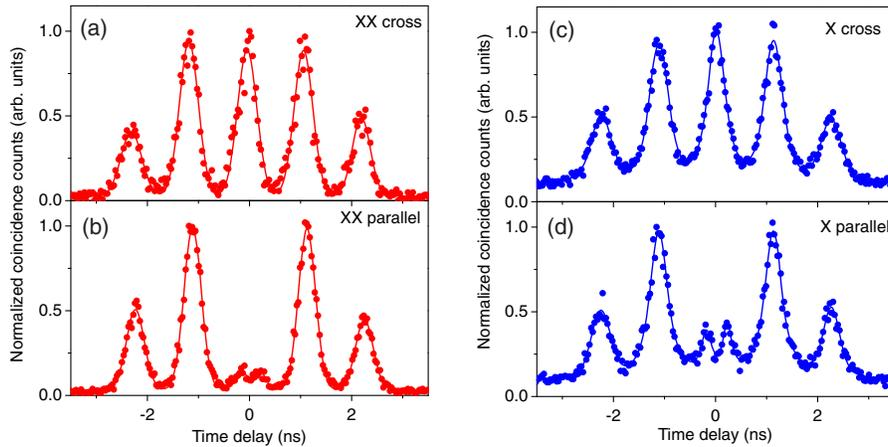
FIG. 4. The interference between two  $XX$  photons is plotted in (a) and (b). The same data for  $X$  photons is shown in (c) and (d). The input two photons are pulse excited and prepared in (a),(c) cross and (b),(d) parallel polarizations, respectively. The fitting function is the convolution of exponential decay (emitter decay response) with Gaussian (photon detection time response). All of the data points presented are raw data without background subtraction.
