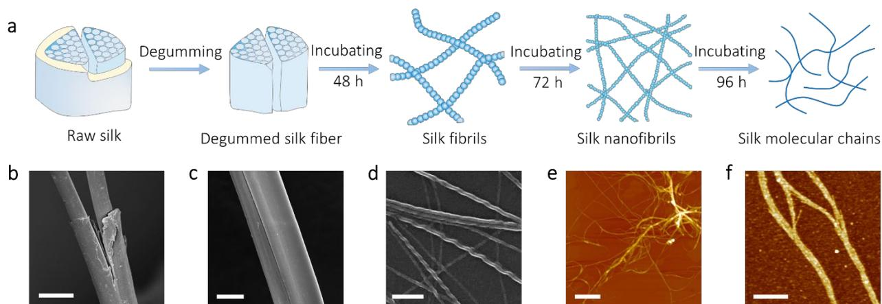
**Figure 1. Exfoliation process for silk fibers and images of silk fibers/fibrils that range from micro to subnano scales.** **a**, Schematic of the process to exfoliate silk fibers from raw silk fiber into silk molecular chains. **b-d**, SEM images of raw silk fiber, degummed silk fiber and silk fibrils. **e-f**, AFM images of silk nanofibrils and silk molecular chains. Scale bars, 10  $\mu\text{m}$  (b), 5  $\mu\text{m}$  (c), 200 nm (d), and 2  $\mu\text{m}$  (e), 500 nm (f).
