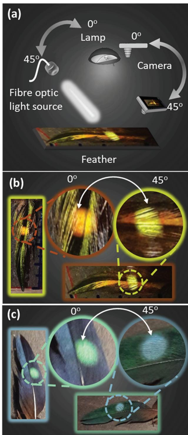
**Figure 4.** Angle-dependent characterization of the feathers. a) Schematic of two-source illumination of the feathers using two interchangeable light sources: a diffused incandescent tungsten lamp and a collimated broadband light to observe two colors at same viewing angle simultaneously. b,c) Photographs of RG and GB feathers taken from two different angles.
