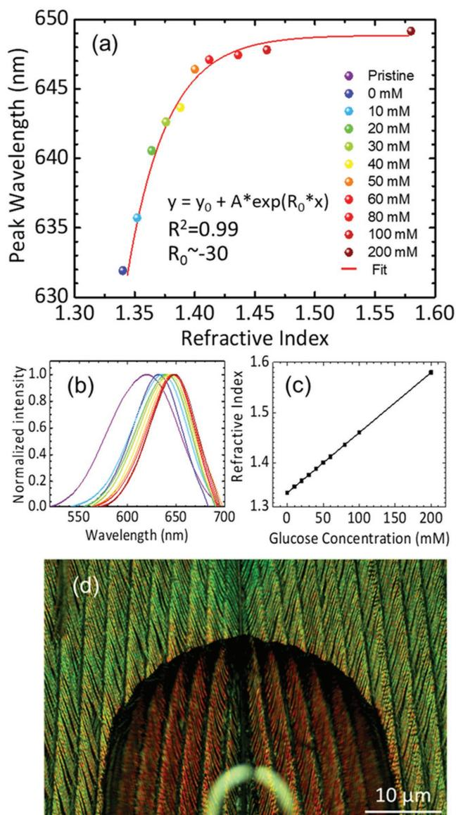
**Figure 7.** Refractive index sensing with Nicobar pigeon's feather. a) Measurement of glucose concentrations from 0 to  $200 \times 10^{-3}$  M. b) Spectral shift with increasing glucose concentration. c) Variation of the refractive index with increasing glucose concentration. d) Visual illustration of glucose sensing under an optical microscope. The feather surface undergoes a redshift upon pouring the glucose solution. The pristine region is unchanged.
