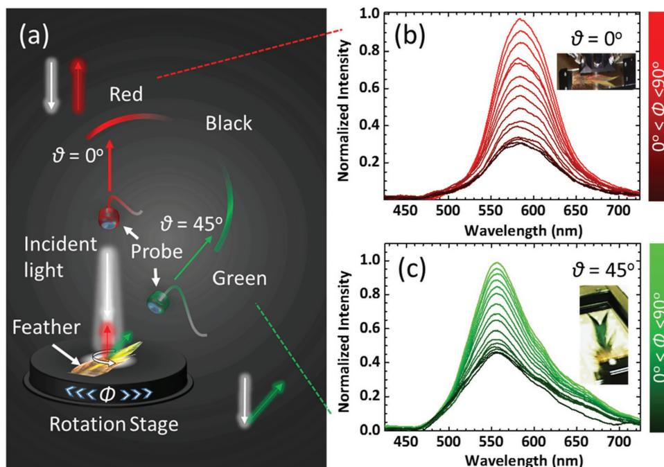
**Figure 3.** Optical characterization of the feathers. a) Schematic for rotational measurement setup. b,c) Variation in optical intensities at  $\theta = 0^\circ$  and  $45^\circ$ , while  $\Phi$  was rotated through  $0^\circ$ – $90^\circ$ .
