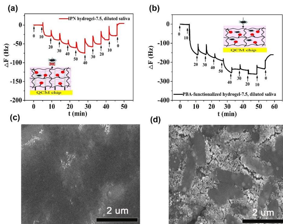
**Fig. 5** (a-b) Response and recovery of glucose in diluted saliva by (a) IPN hydrogel film and (b) PBA-functionalized hydrogel film. The numbers in Fig. 5a and b represent the spiked glucose level. (c-d) SEM images of (c) IPN hydrogel film and (d) PBA-functionalized hydrogel film after 48 h incubation with human saliva.
