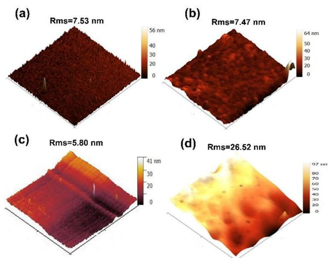
**Fig. 3** AFM images of: (a) uncoated quartz chip; (b) SAM-coated quartz chip; (c) polySBMA brushes-coated quartz chip; and (d) The IPN hydrogel film-coated quartz chip. Different colors indicate different film thickness.
