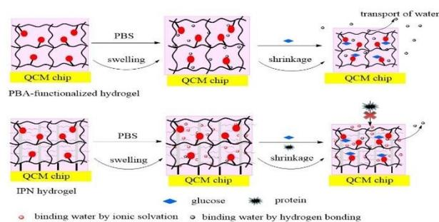
**A stable hydration layer is formed in IPN hydrogel that can achieve the high protein resistance and high glucose sensitivity.**
