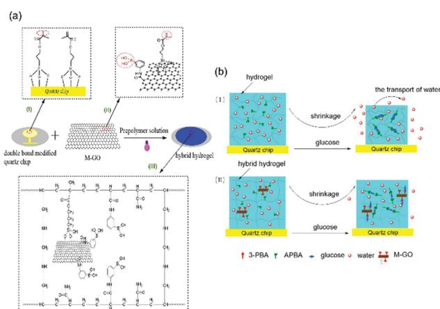
Fig. 1 (a) The synthesis of the hybrid hydrogel-coated QCM sensor, which was obtained by copolymerization of the double bond-modified QCM chip with a rigid M-GO-based monomer and a glucose-sensitive monomer (*i.e.*, 3-APBA); (b) a schematic diagram of the binding of hydrogel and hybrid hydrogel to glucose. Obvious volumetric shrinkage for the hydrogel-coated QCM sensor, while much smaller volumetric change for hybrid hydrogel-coated QCM sensor is observed.
