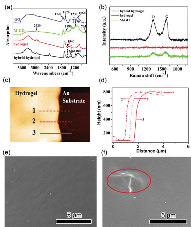
Fig. 2 (a) FTIR spectra of GO, M-GO, hydrogel, hybrid hydrogel; (b) Raman spectra of M-GO, hydrogel, hybrid hydrogel, obtained using a 514 nm excitation wavelength; (c) the AFM image of the hybrid hydrogel film; (d) the thickness of the hybrid hydrogel film. SEM image of (e) hydrogel and (f) hybrid hydrogel.
