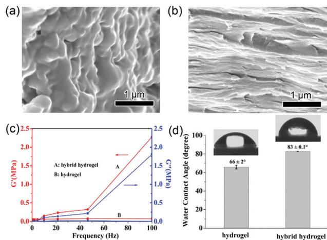
Fig. 4 SEM image of the cross-sectional (a) hydrogel and (b) hybrid hydrogel; (c) storage and loss moduli of the hydrogel and hybrid hydrogel as a function of frequency at room temperature; (d) water contact angles of the hydrogel and hybrid hydrogel.
