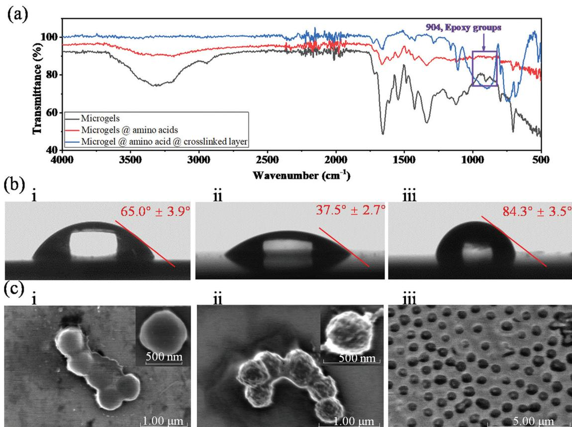
**Fig. 2** (a) FTIR spectra of the synthetic products. (b) Water contact angles of microgels (i), microgels@amino acids (ii), and microgels@amino acid@crosslinked layer (iii). The data indicate the s.d. of three replicating measurements. (c) Microgels had a smooth surface, uniform size, and spherical morphology (i), while the surface of microgels@amino acids was uneven (ii). The microgels@amino acids were wrapped in the crosslinked layer (iii).
