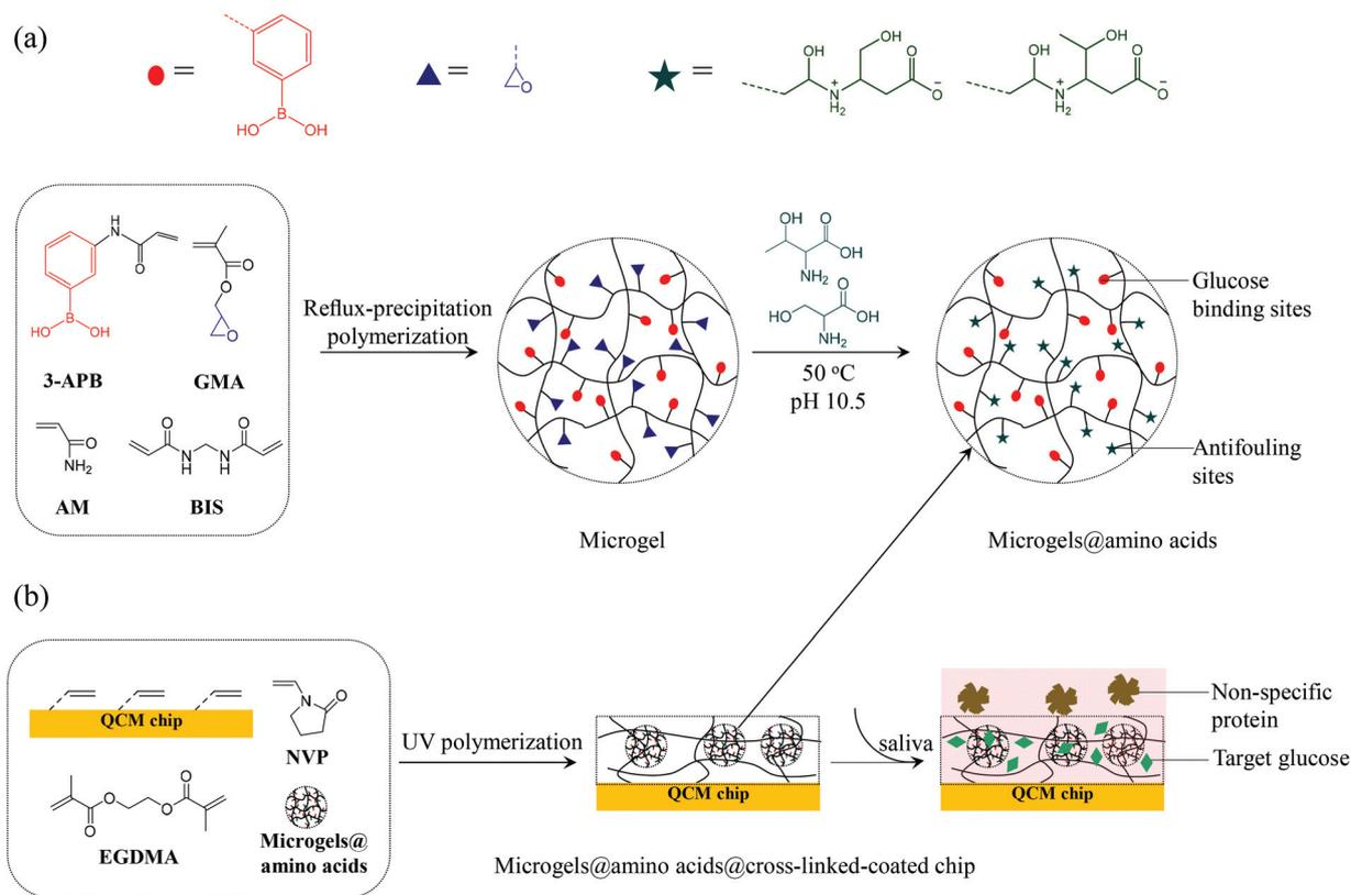
**Fig. 1** (a) Synthesis of microgels through reflux-precipitation polymerization and amino acid grafting onto the surface of microgels by a 'click reaction'. (b) The microgels@amino acids were immobilized on the QCM chip by chemical crosslinking.
